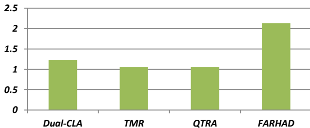
Figure 6. Relative Delay of FARHAD, TMR and Dual-CLA and QTRA compared to CLA adder.
